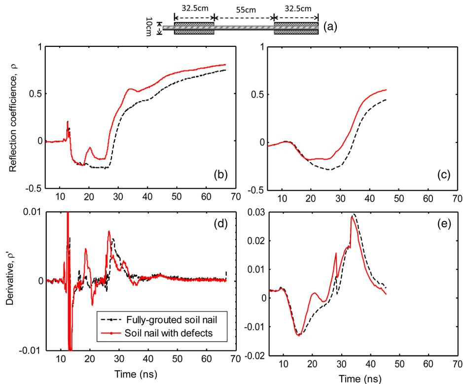
**Fig. 2.** Waveforms of the (a) 1.2-m soil nails with 55 cm defect measured by (b) TDR 100 and (c) TDR 20/20 (fully-grouted soil nails in dotted lines and soil nails with grout defects in solid lines). Corresponding derivative of waveforms are shown in (d) and (e)
