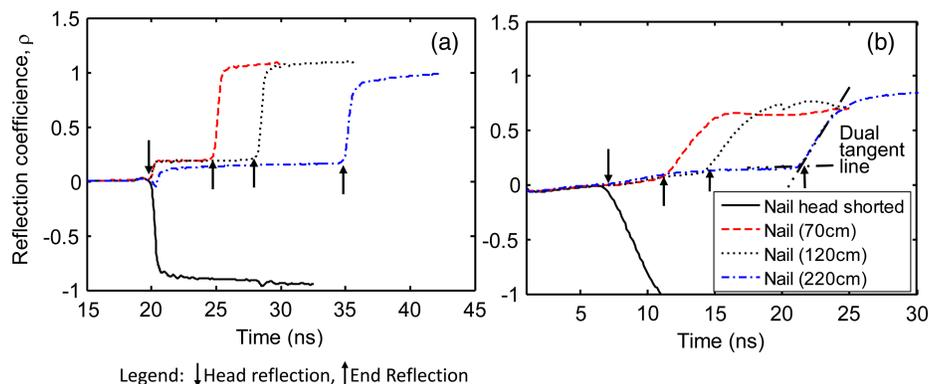
Fig. 1. Measured TDR waveforms on the coaxial cables in the three soil nails of different length using (a) TDR 100; (b) TDR 20/20
